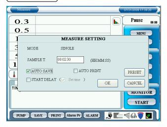
Check "AUTO SAVE" to store data automatically. Check "AUTO PRINT" to print data automatically. Check "START DELAY" to use delay time prior to a measurement.
