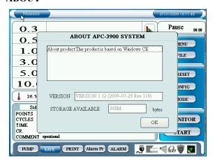
Tap [ABOUT] to view the firmware version of the instrument and remaining capacity of he internal data storage.
