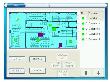
Select a measurement point and tap [START] to start a measurement.
