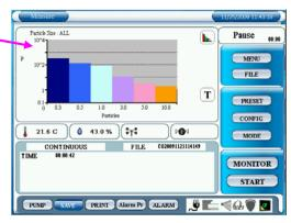
\* After a measurement in REPEAT mode or INTERVAL mode is finished, the measurement result will be displayed.
