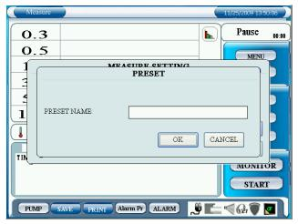
Tap [PRESET] on "MEASURE SETTING" dialog box to display a window asking you to input PRESET NAME.
