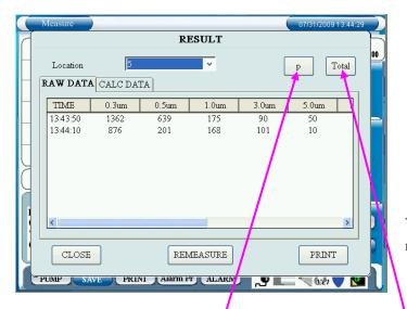
When all of the measurements are finished, a measurement result will be displayed.
