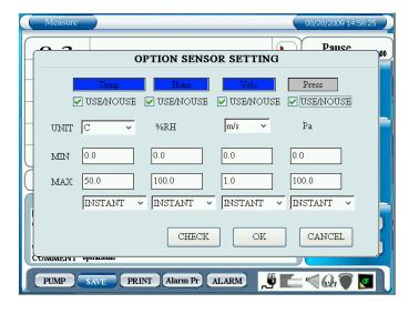
In the OPTION SENSOR SETTING window you can confirm if the option sensor is connected or not, and set to use or not to use the sensor. You can also set the unit and MIN/MAX range value for each sensor. MIN/MAX value should be the spec range for each sensor.
