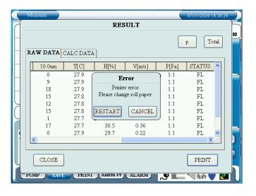
If data cannot be printed out as the printer paper is not installed or some other reasons, the message shown on the left will be displayed.
