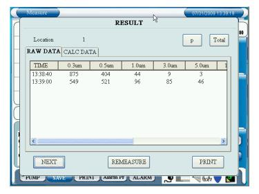
When a measurement at each measurement point is finished, a measurement result window will be displayed each time.
