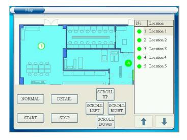
When a MAP is enlarged, [SCROLL UP], [SCROLL DOWN], [SCROLL LEFT] and [SCROLL RIGHT] buttons are activated, which enables you to move MAP.
