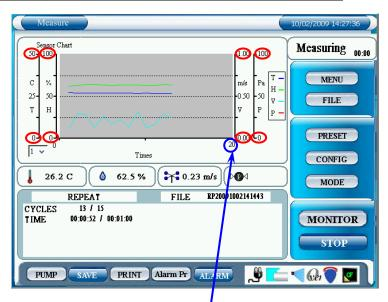
MAX and MIN values set for each sensor in the OPTION tab in the CHART SETTING window is applied in the chart. Tap MAX or MIN value to change it. (It changes in the order of MIN & MAX setting 1, 2, 3.)
