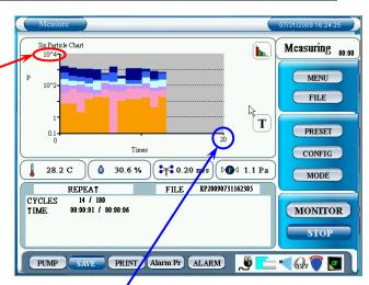
MAX value set in the PARTICLE tab in the CHART SETTING window is applied in the chart.
