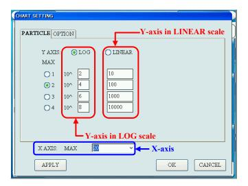
Configure the axis of the chart and range settings. For **X** Axis select either "10", "20", "50", "100", "150" or "300".
