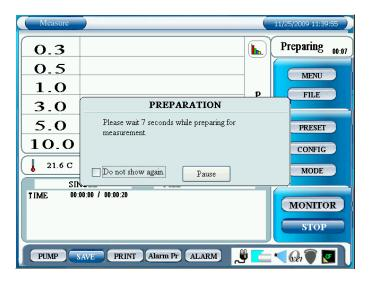
Tap [START] on the main screen to start a measurement in the setting configured in <u>3.5</u> MODE and <u>3.7 CONFIG</u>.
