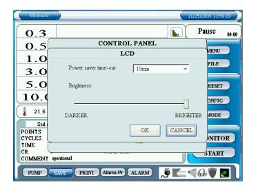
In LCD setting, configure Power saver time-out and Brightness setting.
