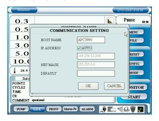
In the COMMUNICATION SETTING, configure the setting for Ethernet connection. This setting shall be configured when connecting the instrument to PC using remote console or remote mode.
