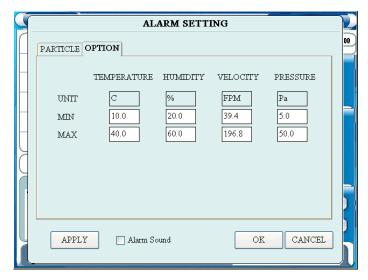
In ALARM SETTING set threshold for particle alarm and option sensor alarm.
