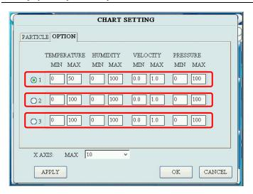
In OPTION tab, configure "MIN" and "MAX" settings for each sensor.
