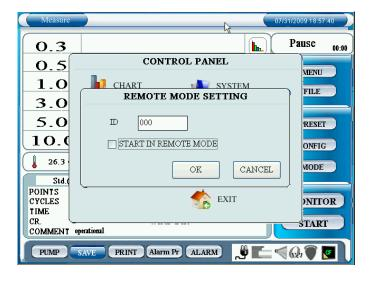
In the REMOTE MODE SETTING, check "START IN REMOTE MODE" to activate remote mode automatically when the instrument is turned ON.
