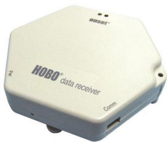
The HOBO data receiver (ZW-RCVR) collects data transmitted from nodes in the ZW series wireless network and uploads it to a computer running HOBOware® 3.0 or later. The receiver forms the network, stores network information, and relays configuration commands to the data nodes. Refer to the *HOBO ZW Series Wireless Network Quick Start Guide* for information on how to set up the receiver.
