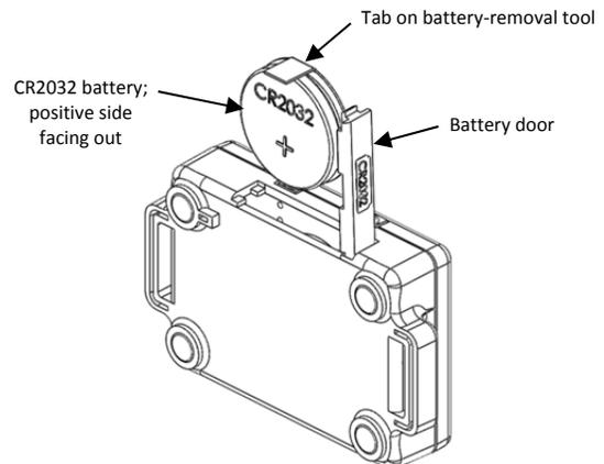
**⚠ WARNING:** Do not cut open, incinerate, heat above 85°C (185°F), or recharge the lithium battery. The battery may explode if the logger is exposed to extreme heat or conditions that could damage or destroy the battery case. Do not dispose of the logger or battery in fire. Do not expose the contents of the battery to water. Dispose of the battery according to local regulations for lithium batteries.
