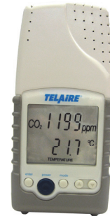
Telaire CO 2 and Temperature Monitor
