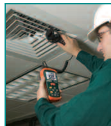
AN100 and AN200 used in HVAC applications measuring airflow from heating vents.
